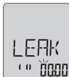
First digit is flashing, EXE increases digit. With STEP to next digit.
