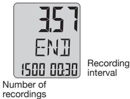
The display END indicates the end of the recording. Activate PREP to return to the PREP-Mode from the END display.
