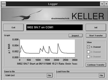
The transfer of the data always starts at the last recording and can be extended to read out the entire memory. The memory may be read out as many times as needed.
