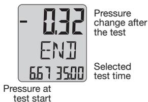
After the test, the measured values are frozen in. Activate PREP to return to the PREP-Mode from the END display.
