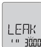
Second digit is flashing, EXE increases digit... With STEP to next digit.
