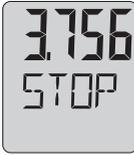
In the STOP mode, a new switch can be connected without influence on status or recording.
